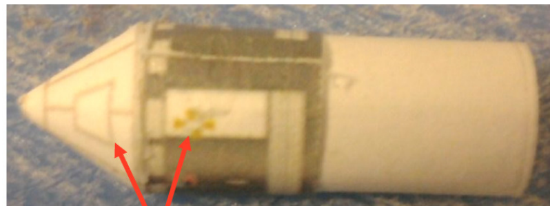
Hatch in line with RCS quad.
