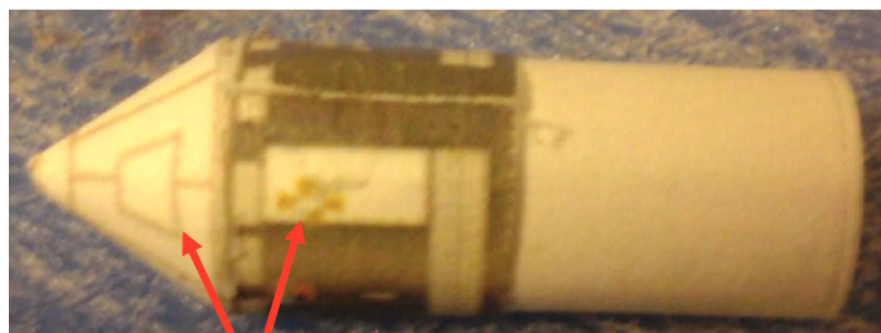
Hatch in line with RCS quad.
