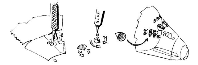
To improve the realism you can cut all the thrusters gray holes and include the nozzles using the parts 1-17 for Vernier thrusters (the small ones) and the 1-18 for the primary thrusters of Reaction Control System. All the nozzles have to be glued inside the part 1-1 with the black side visible through the holes
