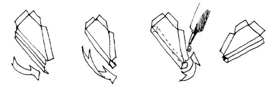
Cut the 8-2 upper part of the aft cargo bay wall. Fold the box spar located in the bottom part of it. Glue it inside the shuttle Engine block.
