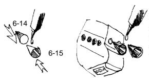
If you want you can cut the holes for the vernier thruster and insert the nozzles 6-16 and 7-16 inside the RCV part. 6-15 and 6-14 are mounted outside to form the two external nozzle of RCS
