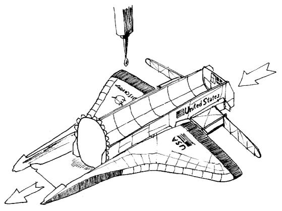
Try to ben both wings in the right shape by leaving weights on them during an entire night. Once the wing stay closed without weight, then insert the cargo bay sliding it from the back side. Glue the wings on the cargo bay tabs. Apply some glue also on the edges of the wing internal structure.
