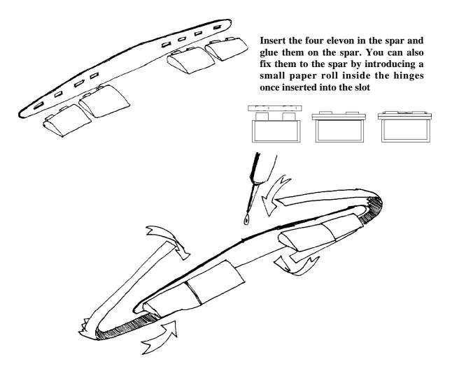
Cut and bend the 6-25 and 7-25. Glue the spar inside it as illustrated. The spar has to be aligned on the centerline. Glue the spar on the painted side, so that the unpainted side stay outside.
