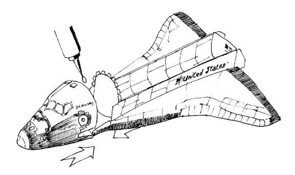
Once the cargo bay and the wings are attached, insert the orbiter fore part and glue it. Try the matching between the part without glue and adjust the tabs before applying the glue.
