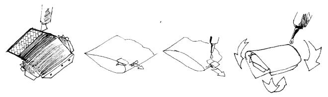
Cut the four elevons 5-10 & 5-11 and the body flap (5-8). Bend and fold them. Cut the hinges 5-9 for the elevons, 5-6 and 5-7 for the body flap. The 5-9, 5-6 and 5-7 have to pass through the slots and glued internally. Once dried, put the glue on the tabs and closes the elevons and flap.
