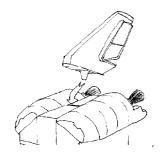
Cut the slot in the upper part of the engine rear block. Glue the red dot marked area and insert the gluing tab of the vertical stabilizer in the slot. Fold and glue the tab inside the rear engine block.
