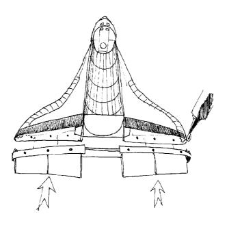
Once it is dried glue the part inside the wing. The spar has to be glued to the cargo-bay lower structure. The gluing tab at the tip are used to glue the black tip of the wings.
