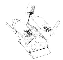
Glue the two OMS pods to the engine block.
