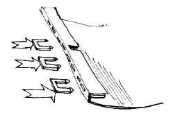
Cut each handle 10-7 fold on the centerline and glue it. Insert each handle in the relative slot (the one corresponding on the right side on the handle). Glue each handle and when you finish glue the back side of part 10-6 on the unpainted part of radiator.
