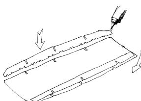
Start with right Thermal Radiator. Cut the radiator 10-5 and the two pieces 10-6 and 10-4 that serve to increase the thickness of the part. Glue them on the back side of radiator 10-5. Cut the three lateral slots carefully on both part. Before to bend cut all the slots for the astronauts handles (the small white boxes on the left edge of the radiator 10-5.
